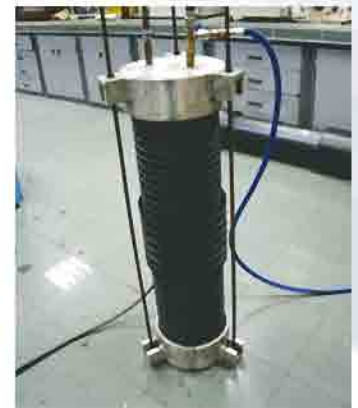
Water Tightness Test
